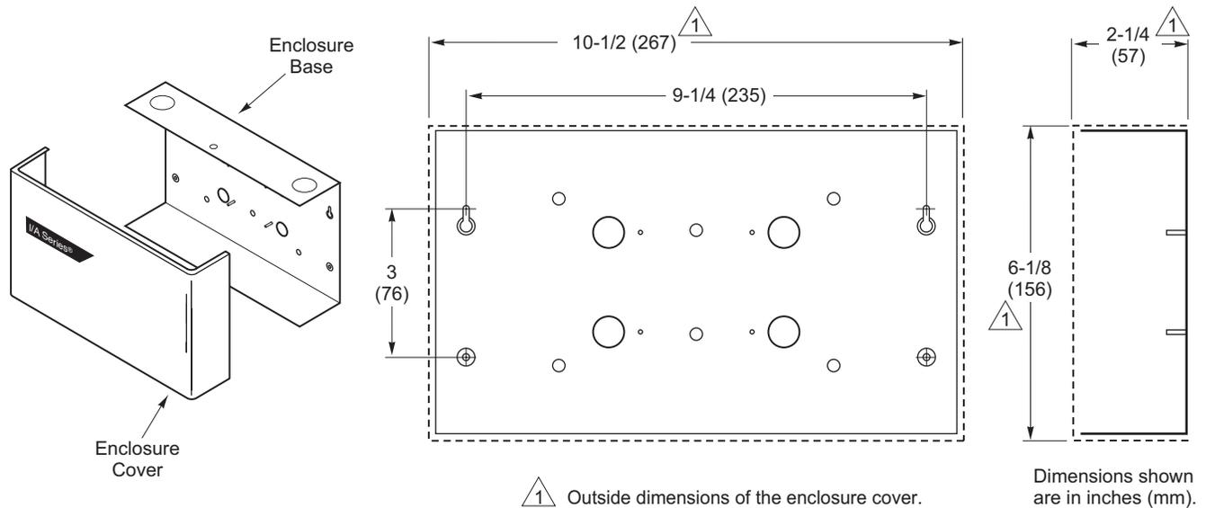
Figure-3 Enclosure MNB-300-ENC Mounting Dimensions.
