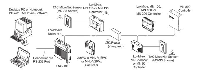
Figure-1 TAC I/A Series MicroNet MN 110 Controller Connectivity.
